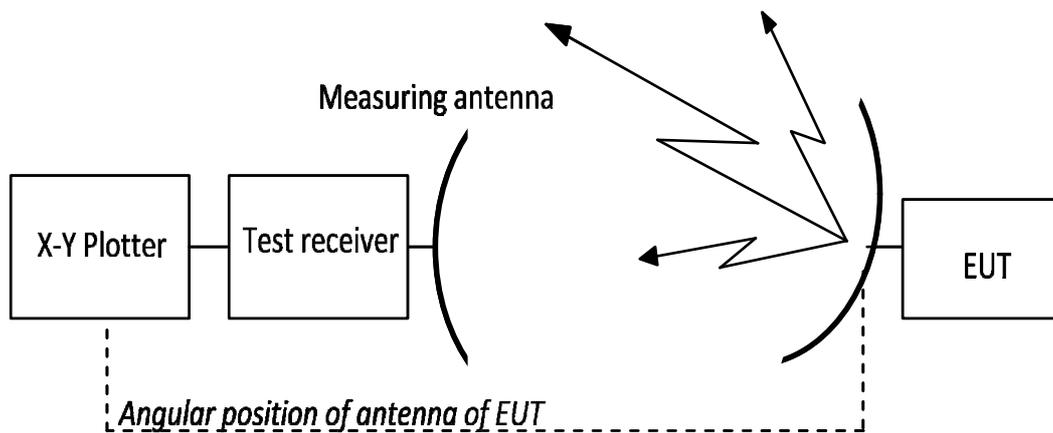
**Figure 8: Test arrangement - antenna beam pointing**
