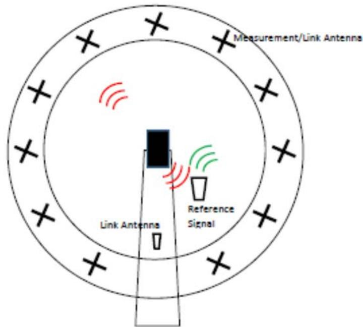
**Figure B.7: Typical NFTF measurement setup**
